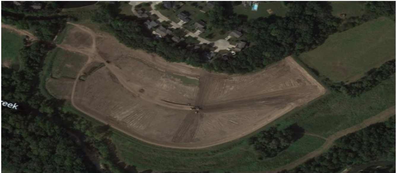
Duello Road Silt Basin. Approximately 22 acres. Our maintenance crew has removed 280K cubic yards of silt from the basin over the last three years in preparation for dredging.
